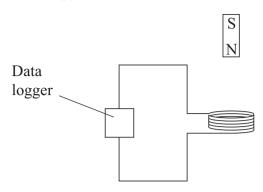
The data from the data logger is used to produce a graph of induced e.m.f. across the coil against time.
